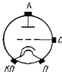
A - anode; C - grid; KP - cathode and heater;
