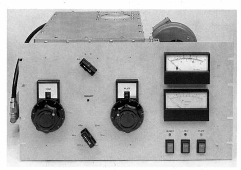
Fig 69—The 3CX1200A7 160- to 10-meter amplifier is built behind a standard 19  $\times$  10½-inch rack panel. Vernier drives are used to control the loading and tuning capacitors. The top meter can be switched to read plate voltage, grid current, forward power and reflected power. (The meter switch is above the LOAD and PLATE dial drives.) The bottom meter is dedicated to plate current. An external low-pass filter is mounted on the left side of the chassis.
