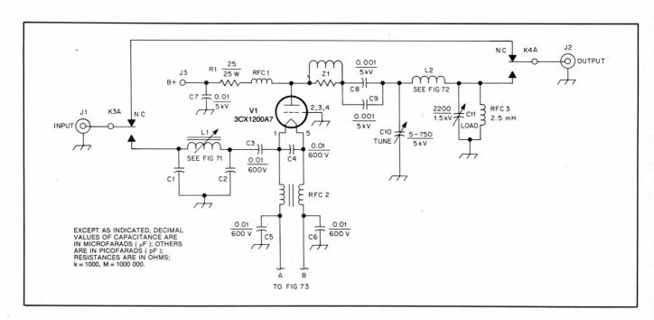
Fig 70—Schematic diagram of the 3CX1200A7 amplifier RF deck. Details of the input and plate-tank circuits are shown in Figs 71 and 72.
