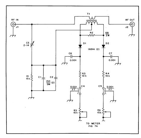
Fig 75—Schematic of the wattmeter circuitry for the 3CX1200A7 amplifier.
