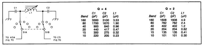
Fig 71—Details of the 3CX1200A7 amplifier input circuit. Component values are shown for Q = 4 and Q = 2. The amplifier was built using the values for Q = 4 (see text).
