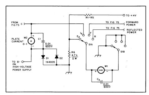
Fig 74—Schematic of the metering circuitry for the 3CX1200A7 amplifier. Note that S1B may be left out and the negative lead from M1 may be returned directly to ground.
