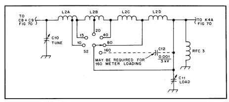
Fig 72—Details of the plate-tank circuit for the 3CX1200A7 amplifier. See Fig 70 for the rest of the circuit.
